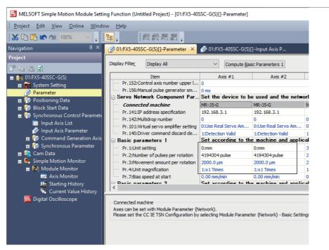
• The basic position information per rotation for the servo amplifier is 26 bit (67108864 pulse).
