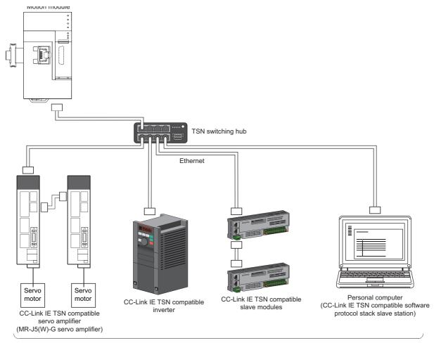
FX5-40SSC-G: Up to 4 Motion control stations + 16 standard stations FX5-80SSC-G: Up to 8 Motion control stations + 16 standard stations
